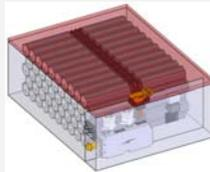
390 V -80kW-17kWh
