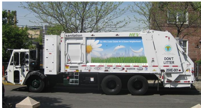
Figure 1: DSNY’s Crane Carrier hybrid-electric refuse truck
