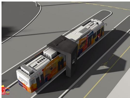
Figure 27: The ABB TOSA articulated electric bus charging at a stop (photo courtesy ABB)
