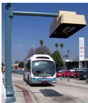
Figure 10: The Proterra EcoRide BE35 (left) and deployed super-fast charger (right)
