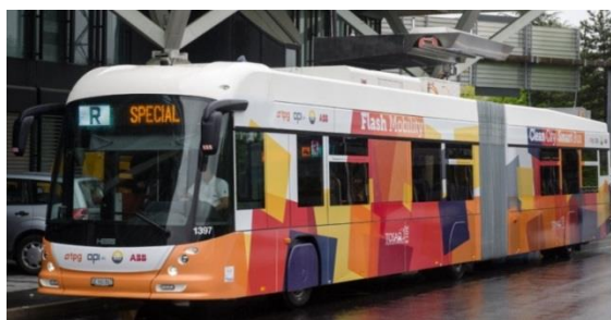
Figure 2: The ABB TOSA articulated electric bus charging at a stop (photo courtesy ABB)
