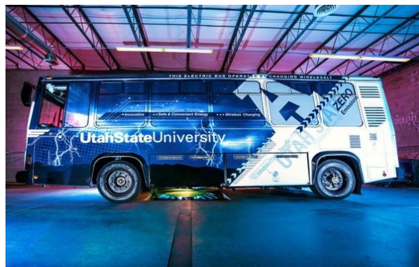
Figure 25: Shuttle bus powered by WAVE technology (photo courtesy Utah State University)
