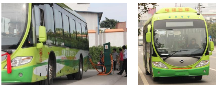
Figure 6: The Hengtong electric bus charging (left) and en-route (right) (photo courtesy en.htebus.com)
