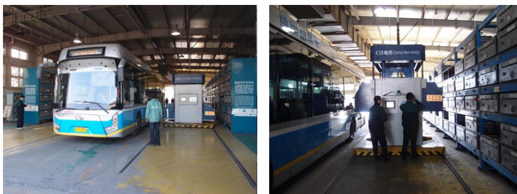
Figure 26: Battery swapping system in Beijing, China
