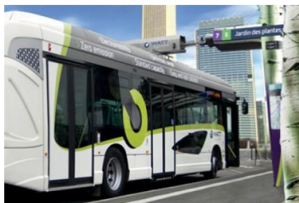
Figure 8: PVI Watt system with deployed charging arm (photo courtesy busworld.org)
