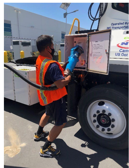
Figure 59: Transpower Charging Connector for Kalmar Electric Yard Tractors at NFI
