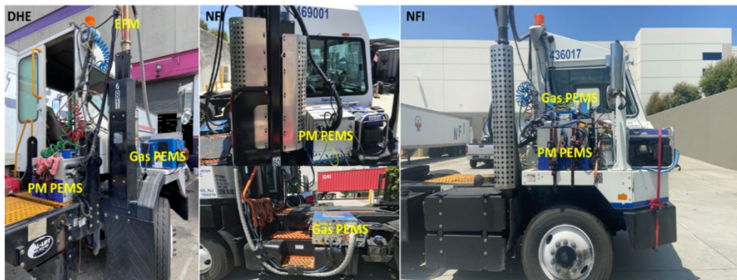
Figure 76: PEMS Equipment Installed on Diesel Yard Tractor
