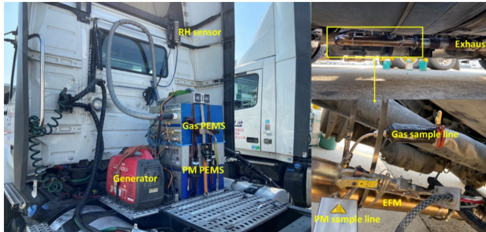
Figure 75: PEMS Equipment Installed on Diesel Box Truck
