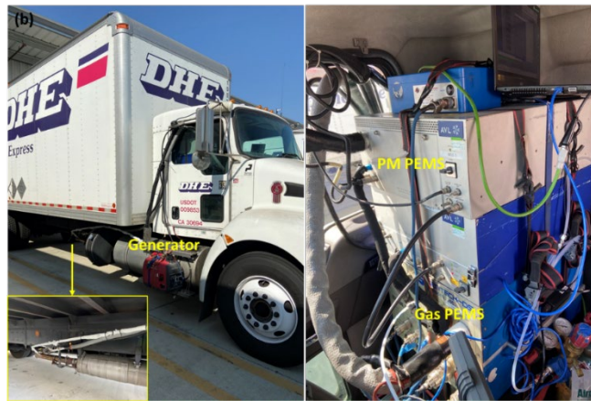
Figure 76: PEMS Equipment Installed on Diesel Yard Tractor
